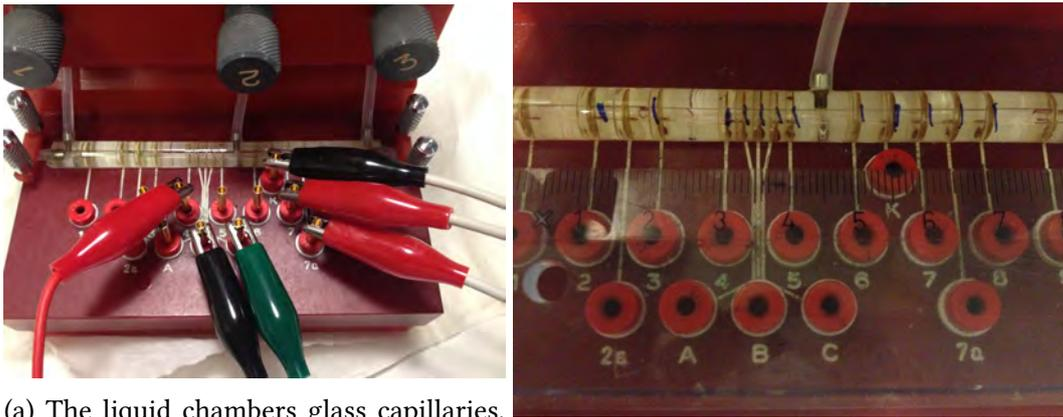
(a) The liquid chambers glass capillaries, with the three injections sites, the recording electrodes and the stimulation electrodes. (b) The liquid chamber, finding the distance between the stimulation and the recording electrodes.
